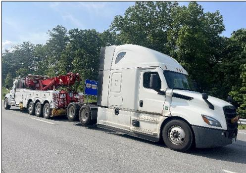
The towing and recovery of heavy-duty vehicles like Class 8 tractor-trailers requires specialized heavy-duty equipment that is not required for the day-to-day operations of most T&R companies. The most important of these is a heavy-duty wrecker. Wreckers are equipped with a boom and a wheel lift that can maneuver heavy-duty vehicles as well as tow them. Most wreckers have a capacity between 25 and 50 tons (50,000 to 100,000 lbs.).
